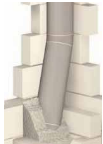
Typical offset using 2 liner bends and a 200L600 mm straight liner
